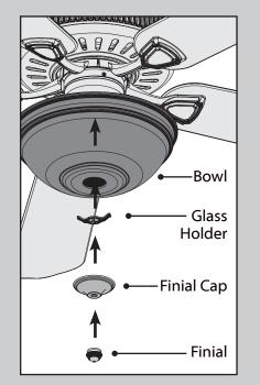
Press the bowl and glass holder flush against the metal plate. Thread the light pull chain through the hole in the center of the finial cap and thread the fan pull chain through the grommet hole in the side of the finial cap.
